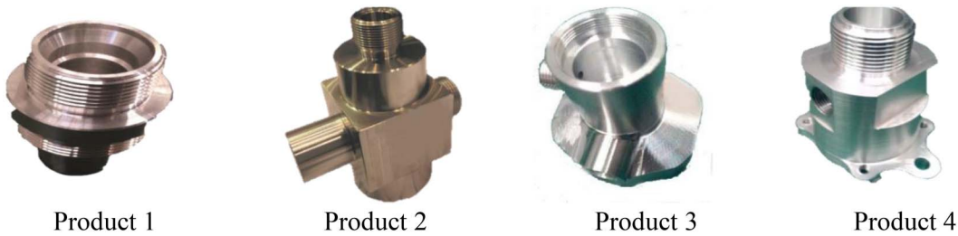
Fig. 5. Four types of products manufactured by the multistage system.
